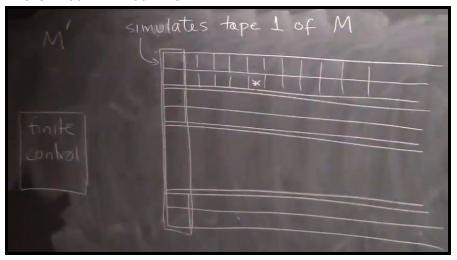
It will have one tape, but divided up into 2k tracks. It will have 2 tracks for each tape in M. In other words, every 2 tracks in M' corresponds to 1 tape in M. The first track in every pair of tracks will simulate the corresponding tape of M. The second track in every pair of tracks is blank everywhere, except for in 1 square, where it has a star. That star represents the location of the tape head of the corresponding tape in M.
