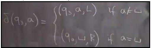
I.e. If a is not the blank symbol, then we keep moving left. If a is the blank symbol, we enter state Q0 and move 1 cell to the right.
