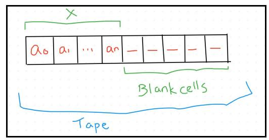
The input string, x, is not allowed to contain any blank cells. This is because for the TM to determine the end of the input, it starts from the leftmost cell and goes to the right until it hits a blank cell. If the input itself contains a blank cell, then the TM would never know when the input ends.
