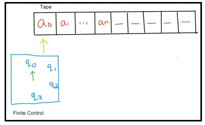
Given its current state and the input, the TM either changes state or changes the input and it moves to the left or the right. The TM keeps executing these steps until the state that it's in becomes one of two special states, **Qa** or **Qr**.
