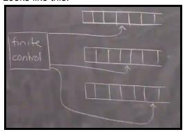
There is one control machine and there are k tapes. Each of these k tapes has its own tape head.
